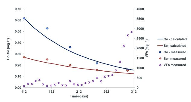
Figure 1 Cobalt and selenium dilute out curves in the pair of digesters where Se, Mo, Co, W, Fe, and Ni supplementation ceased on day 112. (By day 245 the VFA concentration in the digesters had risen above 500 mg  $l^{-1}$ .)
